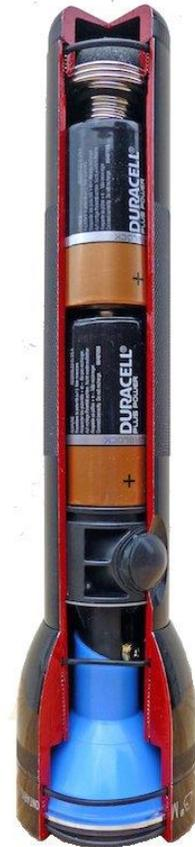
When batteries or solar cells are connected in series, the voltage is added. So, in the example of our flashlight, the two 1.5 volt D-cell batteries are providing a total of 3.0 volts of power to the flashlight. If we had a three battery flashlight (3 cell) it would be providing 4.5 volts of electrical power.
