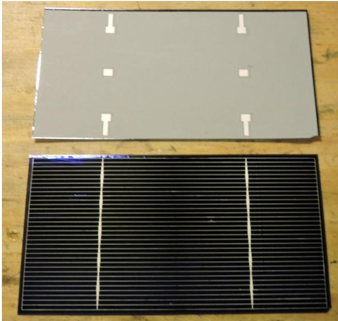
To start, tabbing wire needs to be attached to the negative side of the solar cell. Tabbing wire is a 2mm wide, flat, uninsulated wire. It is silver colored when you buy it, because it is already coated in solder, in a process called "tinning."
