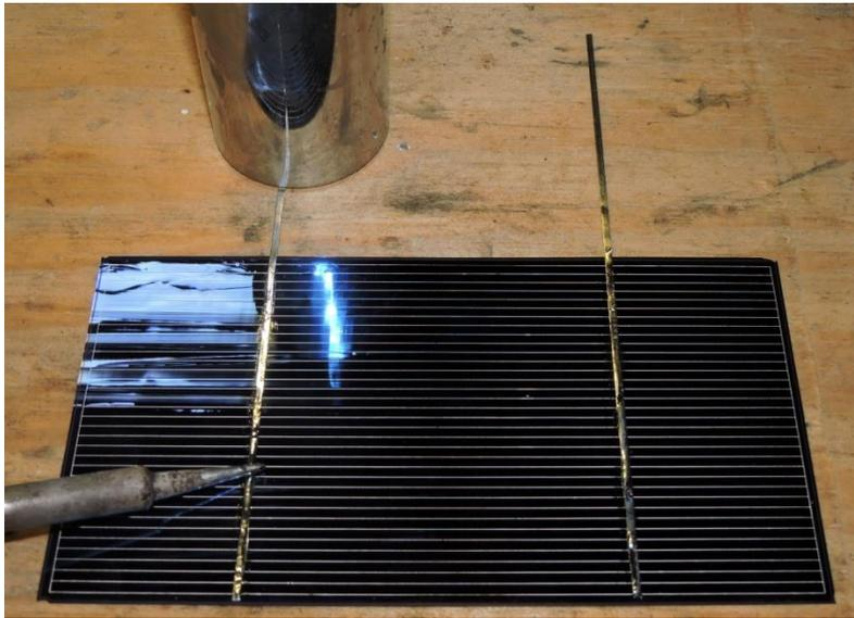
Before soldering the tabbing wire onto the cell, take the flux pen and put a line of flux down both of the solder pads. To get the flux flowing in the pen, you'll need to push down on it on some hard surface. Don't try pushing on it on a solar cell, or it will break the cell.
