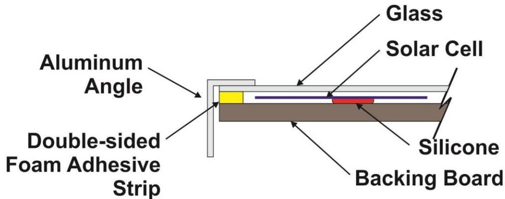
Measure the thickness of your foam adhesive stripping and compare it to the height of the cells off the top of your backing panel. If they are higher than the thickness of the strip, you'll need to use two layers of it, rather than one. So, whenever I talk about using it, use double.
