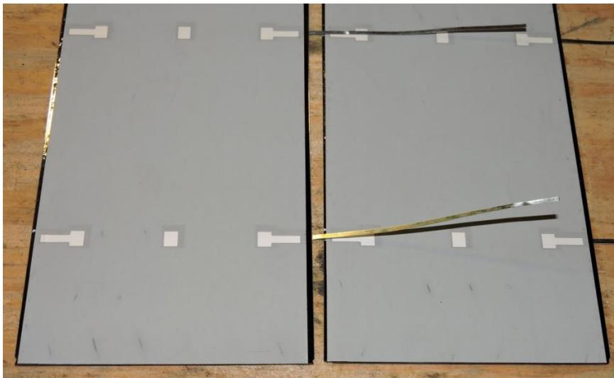
I'd also recommend using a straight edge, attached to your workbench top, so that you can make sure that you are aligning the cells in a straight string. If they are not straight, you may have trouble when you try and fit the strings together to make a solar panel out of them.
